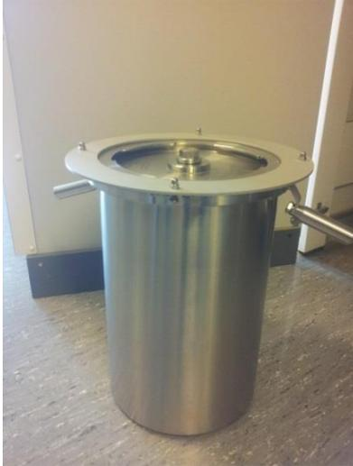
There are a number of special DPTE containers in use in some places. These can be connected to the bottom plate of a class III cabinet. Procedures (using, closing, transport) relating to these DPTE containers, are known and managed by the organisations that work with them.
