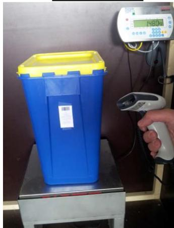
A WIVA container is a blue container with a yellow lid, has a 30 or 60 litre capacity and a biohazard sign. Once closed this container can no longer be opened and is suitable for the disposal of waste with:
