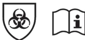
If protection is (also) required against skin contact from **viruses**, the suitability of the glove can be identified by the following symbol on the packaging:
