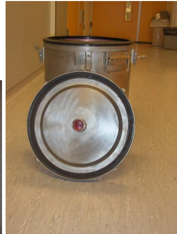
Lid stainless-steel container underside (silicone rubber rim and colored pop-up cap)
